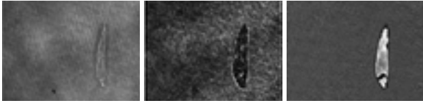
(Left) Example of digital hologram of Euglena Acus , (center) intensity and (right) unwrapped phase reconstruction of the wavefront.
