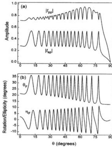
**Figure 4.** A p-polarized plane wave ( $\lambda = 550$  nm) is incident at oblique angle  $\theta$  on a  $20\text{ }\mu\text{m}$ -thick slab, as shown in Figure 2(b). The slab ( $\epsilon = 5.5$ ,  $\epsilon' = 0.01i$ ) is magnetized along the Z-axis. (a) Plots of  $|t_{pp}|$  and  $|t_{sp}|$ , the transmitted polarization components along the p- and s-directions, as functions of  $\theta$ . (b) Plots of  $\theta_F$  and  $\eta_F$  versus  $\theta$ .
