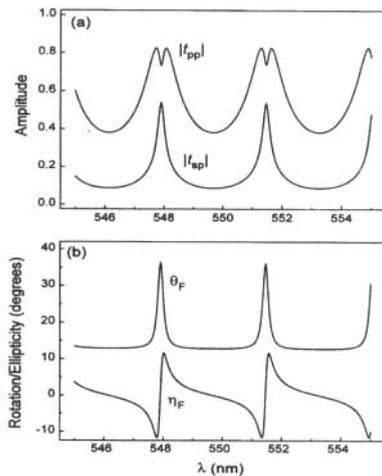
**Figure 5.** A p-polarized plane wave is incident at  $\theta = 85^\circ$  on the slab described in Figure 4. (a) Plots of  $|t_{pp}|$  and  $|t_{sp}|$ , the transmitted p- and s-components of polarization, as functions of  $\lambda$ . (b) Plots of  $\theta_F$  and  $\eta_F$  versus  $\lambda$ .
