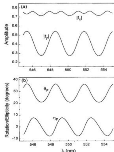
**Figure 3.** A plane wave, linearly polarized along the X-axis, is normally incident on a 20  $\mu\text{m}$ -thick slab, as shown in Figure 2(a). The slab ( $\varepsilon = 5.5$ ,  $\varepsilon' = 0.01i$ ) is magnetized along the Z-axis. (a) Plots of  $|t_x|$  and  $|t_y|$ , the transmitted polarization components along the X- and Y-axes, as functions of  $\lambda$ . (b) Plots of polarization rotation angle  $\theta_F$  and ellipticity  $\eta_F$  versus  $\lambda$ .
