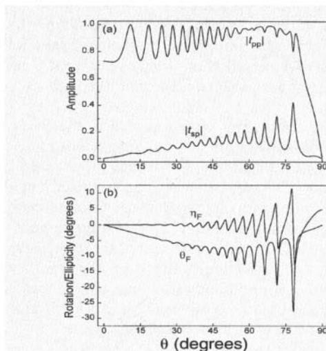
**Figure 10.** Longitudinal Faraday effect, arising when a p-polarized plane wave ( $\lambda = 550$  nm) is incident at oblique angle  $\theta$  on a  $20\ \mu\text{m}$ -thick slab. The slab ( $\epsilon = 5.5$ ,  $\epsilon' = 0.01i$ ) is magnetized along the X-axis, as depicted in Figure 9(a). (a) Transmitted amplitudes  $|t_{pp}|$  and  $|t_{sp}|$  versus  $\theta$ . (b) Polarization rotation angle  $\theta_F$  and ellipticity  $\eta_F$  versus  $\theta$ .
