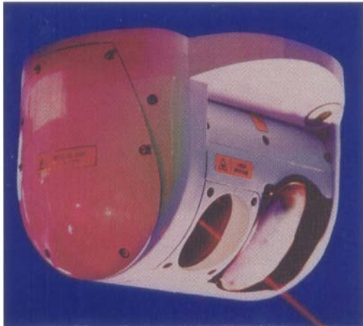
Figure 2. The Nemesis system protects aircraft from infrared-guided surface-to-air missiles.
