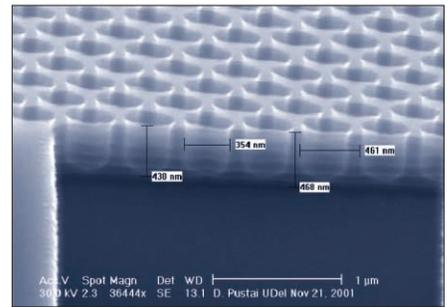
**Figure 4.** Scanning electron microscope image of a triangular photonic crystal lattice etched into a 450-nm-thick device layer SOI wafer.
