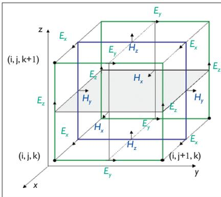
**Figure 2.** Illustration of the computational domain of the FDTD method.
