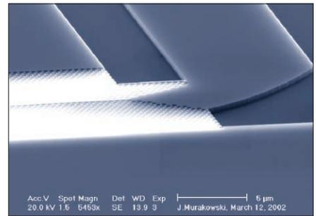
**Figure 7.** Scanning electron microscope image of a fabricated J-coupler.
