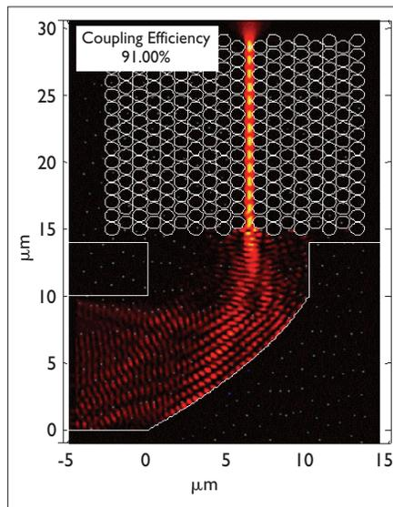
**Figure 6.** Simulation of a parabolic coupling structure for coupling from a 10- $\mu\text{m}$ -wide silicon waveguide into a single-defect photonic crystal device.
