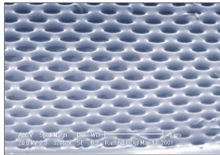
**Figure 3.** Scanning electron microscope image of a triangular photonic crystal lattice in PMMA.
