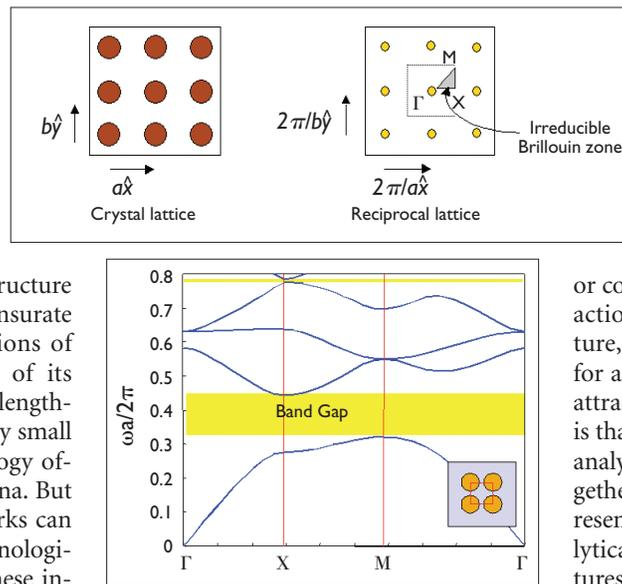
**Figure 1.** (a) Diagram of a 2D rectangular lattice and its representation in the reciprocal space, and (b) dispersion diagram of a rectangular lattice
