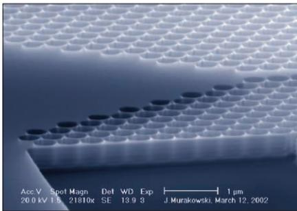
**Figure 5.** Scanning electron microscope image of an etched, high-fill-factor photonic crystal lattice that serves to illustrate the potential of a sequential etch process.
