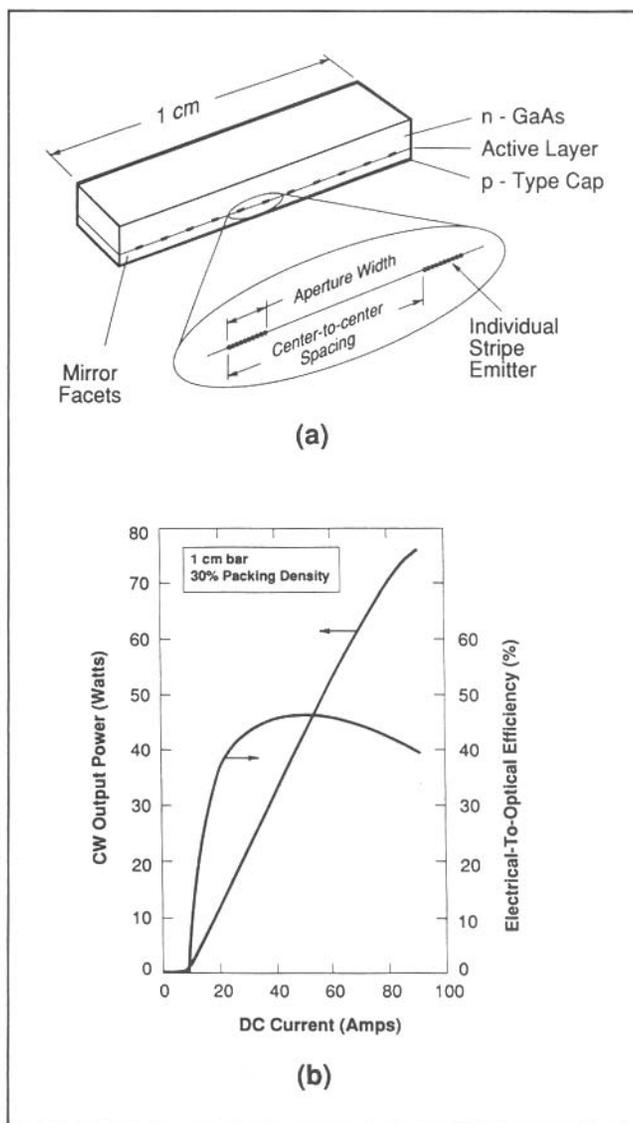
(a) Schematic diagram of a monolithic laser diode array structure. (b) Output power vs. current for a high power cw laser with a thirty 10-stripe structure (30% packing density) at 0° C heatsink temperature.
