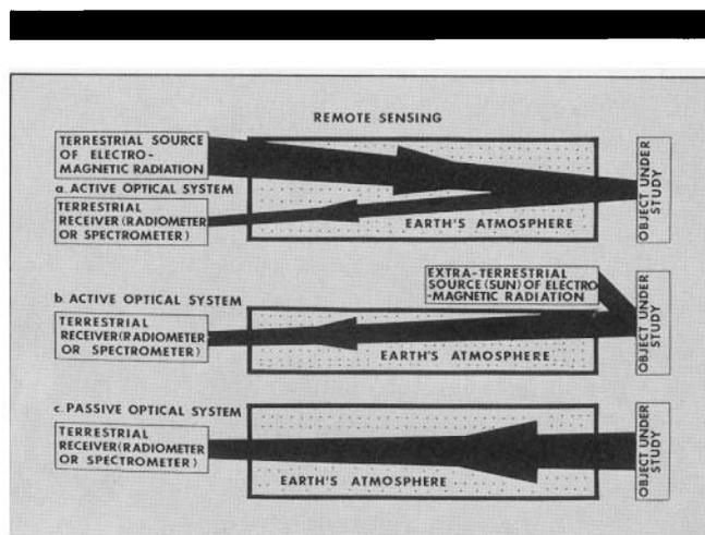
FIGURE 1. Active versus passive optical systems for carrying out remote sensing (or remote sampling).
