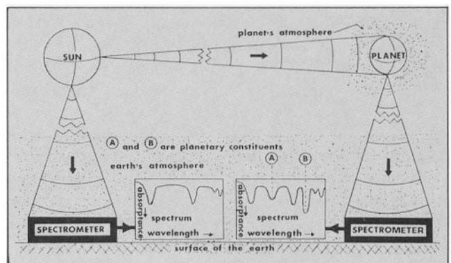
FIGURE 4. Determining the constituents in a planet's atmosphere.
