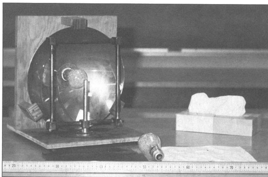
**FIGURE 1.** Kleenex, concave mirror, and flashbulb apparatus used by the author to demonstrate that electromagnetic radiation possesses energy.
