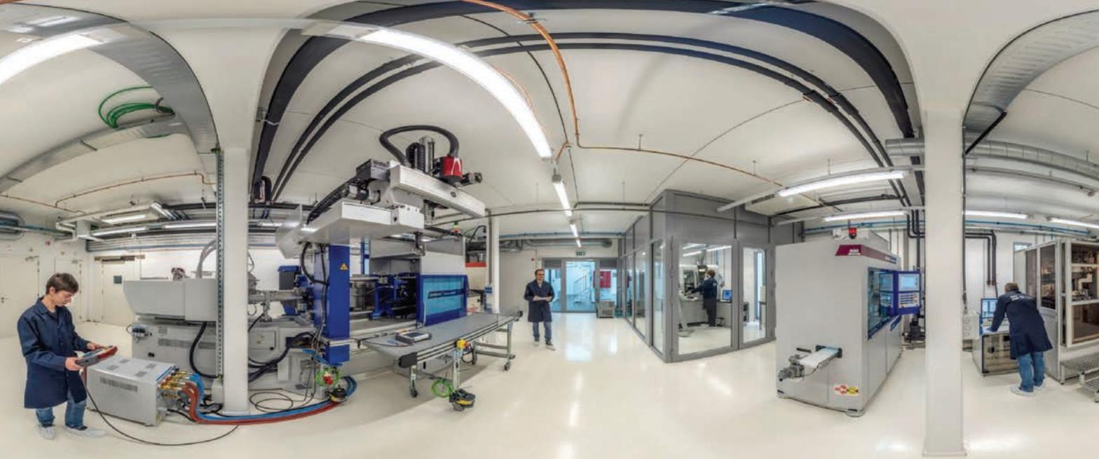
One of the “Experience Centers” run by PhotonHub Europe, focused on fabrication, offers hands-on training with injection and glass-press molding, diamond tooling and hot-embossing equipment.
