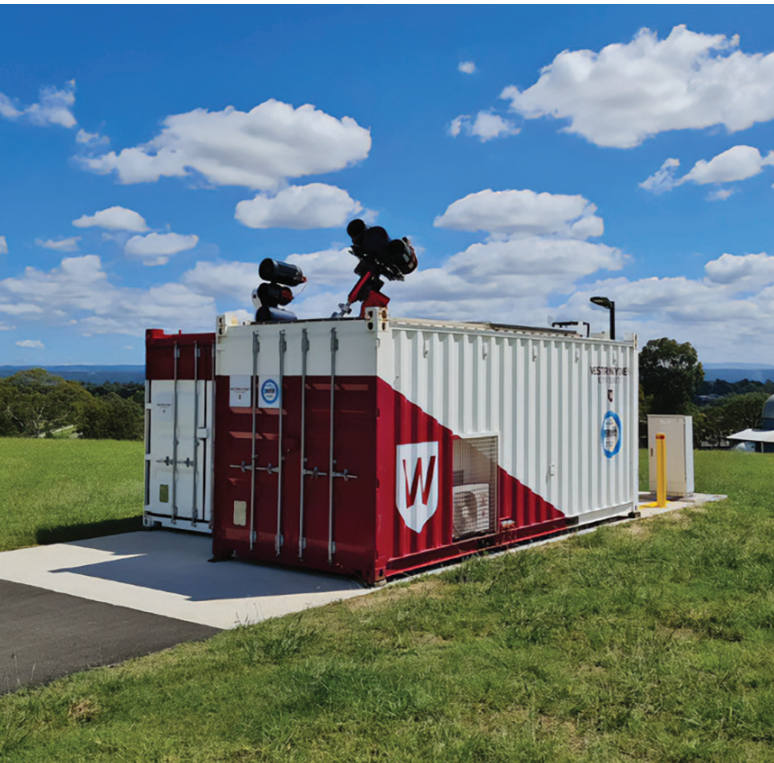
A photo of Astrosite, a mobile observatory built by Greg Cohen and colleagues that fits inside a shipping container. The high dynamic range of an event camera allows the observatory to operate day or night. International Centre for Neuromorphic Systems, Western Sydney University
