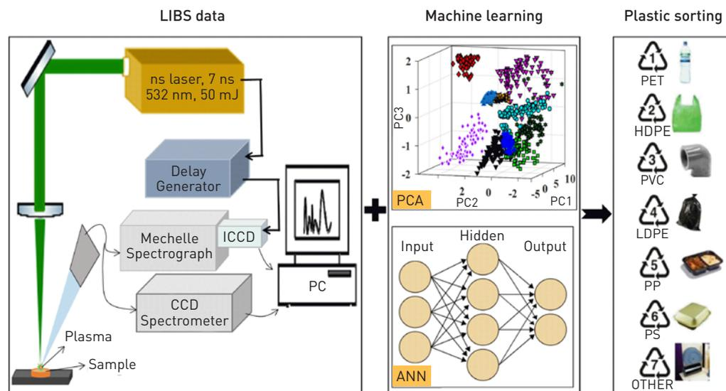
In the recently demonstrated system, data from a typical LIBS experimental setup (left) undergoes principal-component analysis (PCA) and artificial neural network (ANN) analysis (center), enabling identification and sorting of plastic waste (right).
